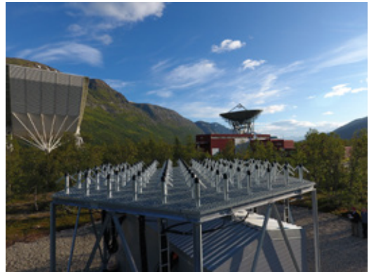
EISCAT 3D test array on the EISCAT site in Tromsø. Photo: Craig Heinselman Heinselman
